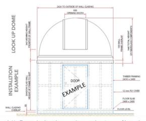
The Look Up Dome is placed on a unique and waterproof base ring design which enables the dome to be fitted to any square opening 2.42metres (2420mm) across.
